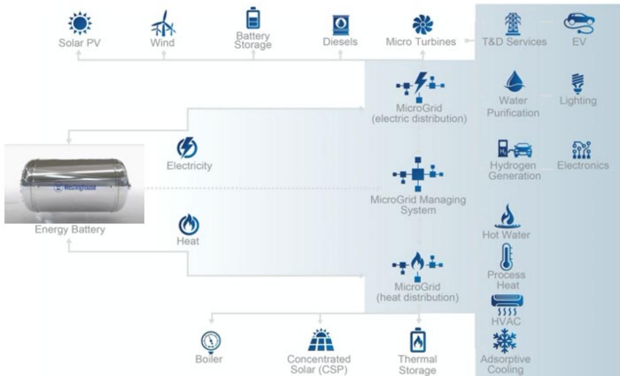
**Figure 3 eVinci Reactor Module Energy Products**
