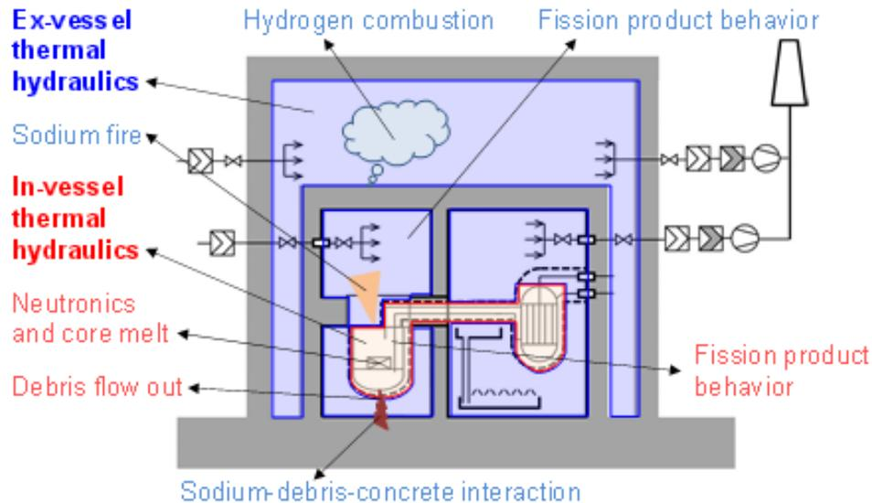
**Figure 1. Physical models to be integrated into SPECTRA**
