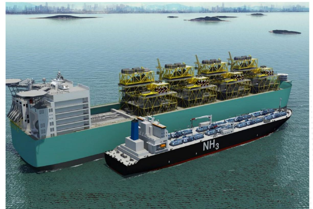
Figure 15- 3. Conceptual ammonia bunker offloading ammonia from a production platform. Lucid Catalyst Graphic.
