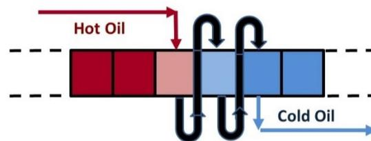
**Figure 2. Sequential heating of crushed rock bed with hot oil**
