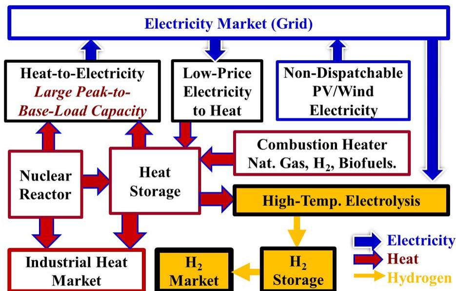
**Figure 1. Base load nuclear, wind, and solar with heat storage to provide variable heat, electricity, and hydrogen**
