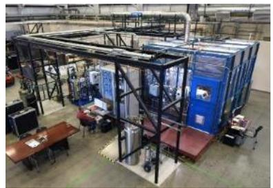
25 kW high-temperature electrolysis @ INL Energy Systems Laboratory
