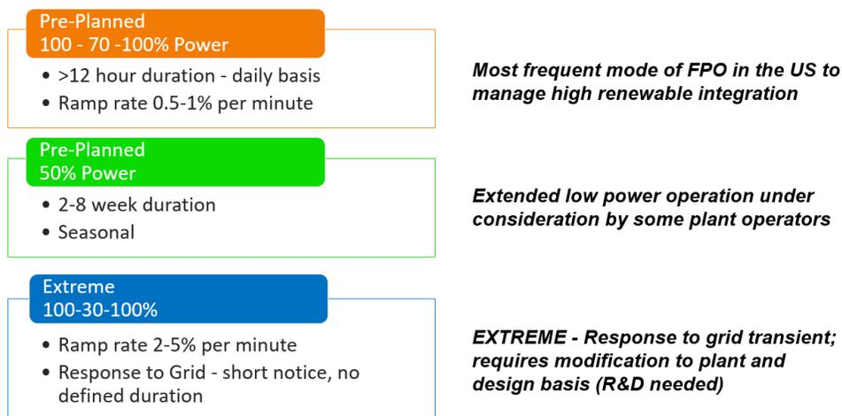
**Figure 1 Categorization of Flexible Operations for Nuclear Power Plants in the United States by Ramping Requirements, Frequency, and Duration.**
