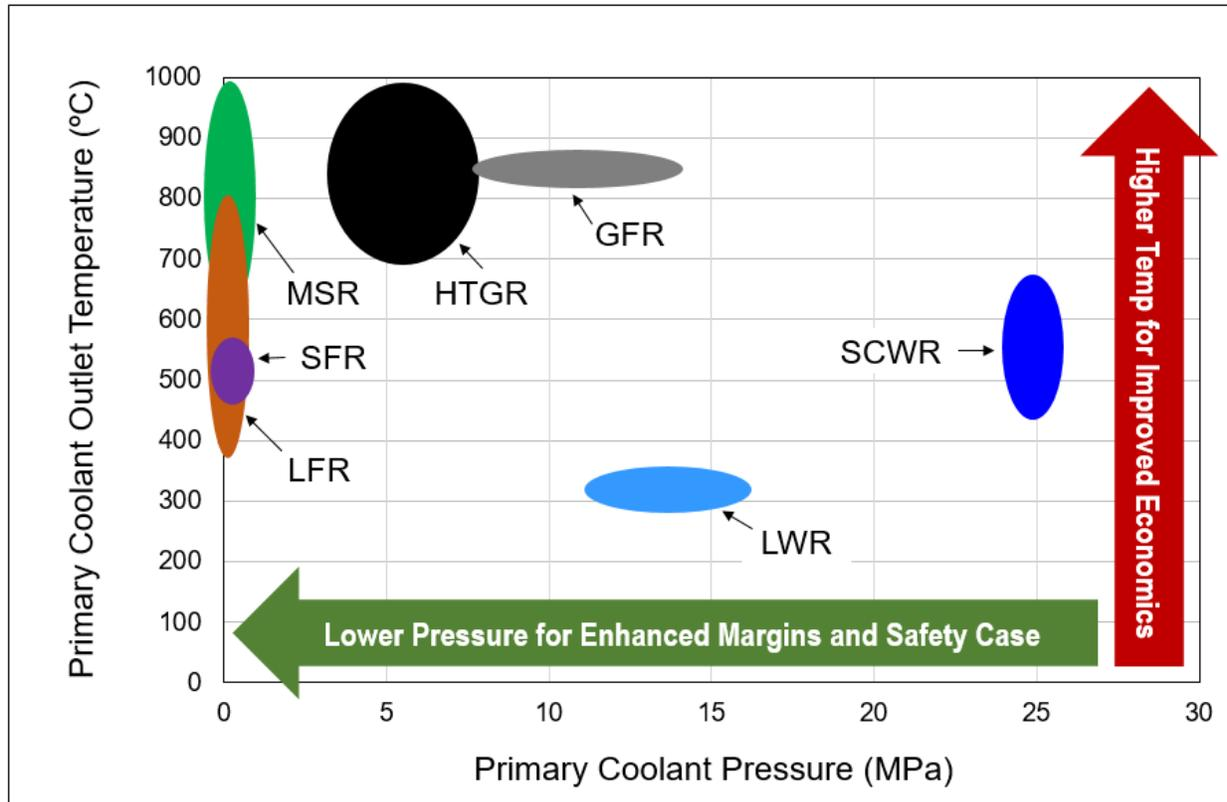
**Figure 2 Primary coolant outlet temperature vs. pressure for current and advanced reactors.**
