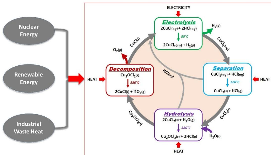
**Figure 4. Hybrid Cu-Cl thermochemical hydrogen production**
