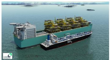
Figure 3. Conceptual ammonia bunker offloading ammonia from a production platform.
