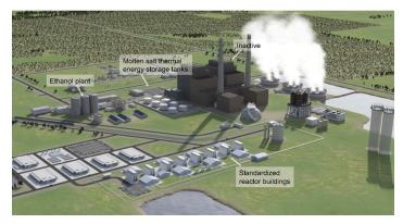
Figure 1. Repowering coal case study: two-steam-unit, 1,200 MWe plant<sup>5</sup>
